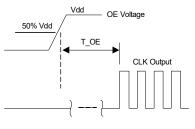
T\_OE: Time to re-enable the clock output
