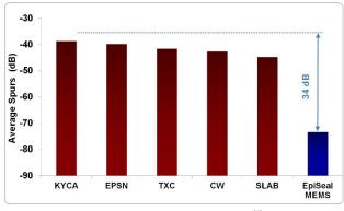
Figure 5. Vibration Robustness<sup>[5]</sup>
