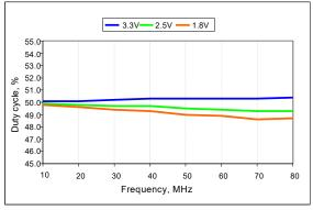
Figure 10. Duty Cycle vs Frequency
