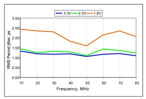
Figure 9. RMS Period Jitter vs Frequency
