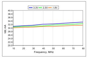
Figure 8. Idd vs Frequency
