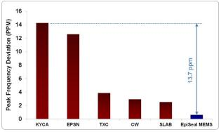
Figure 4. Power Supply Noise Rejection<sup>[4]</sup>
