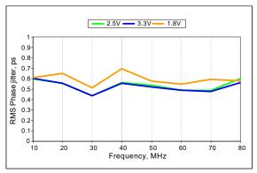
Figure 11. RMS Phase Jitter vs Frequency
