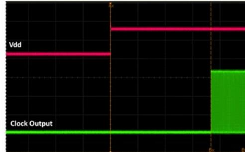
**Figure 16. Startup Waveform vs. Vdd**
