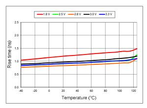
Figure 11. 20%-80% Rise Time vs Temperature
