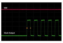
Figure 17. Startup Waveform vs. Vdd (Zoomed-in View of Figure 16)
