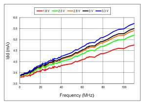
Figure 7. Idd vs Frequency
