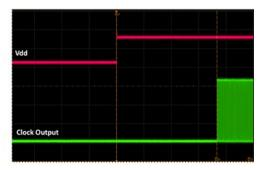
Figure 16. Startup Waveform vs. Vdd
