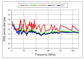
Figure 9. RMS Period Jitter vs Frequency
