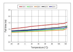
Figure 12. 20%-80% Fall Time vs Temperature
