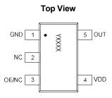
Figure 1. Pin Assignments
