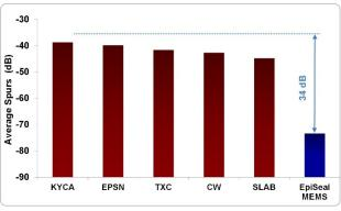
Figure 5. Vibration Robustness<sup>[5]</sup>
