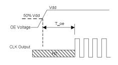
T\_oe: Time to re-enable the clock output
