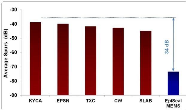
Figure 5. Vibration Robustness<sup>[5]</sup>
