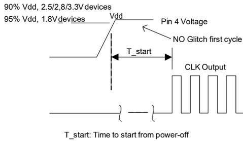
Figure 4. Startup Timing (OE/ $\overline{\text{ST}}$  Mode)
