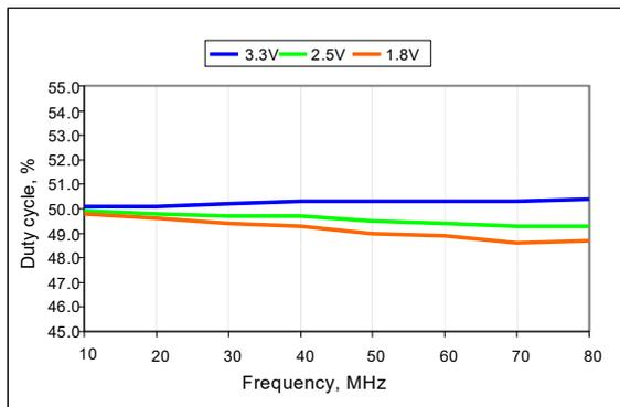
Figure 10. Duty Cycle vs Frequency
