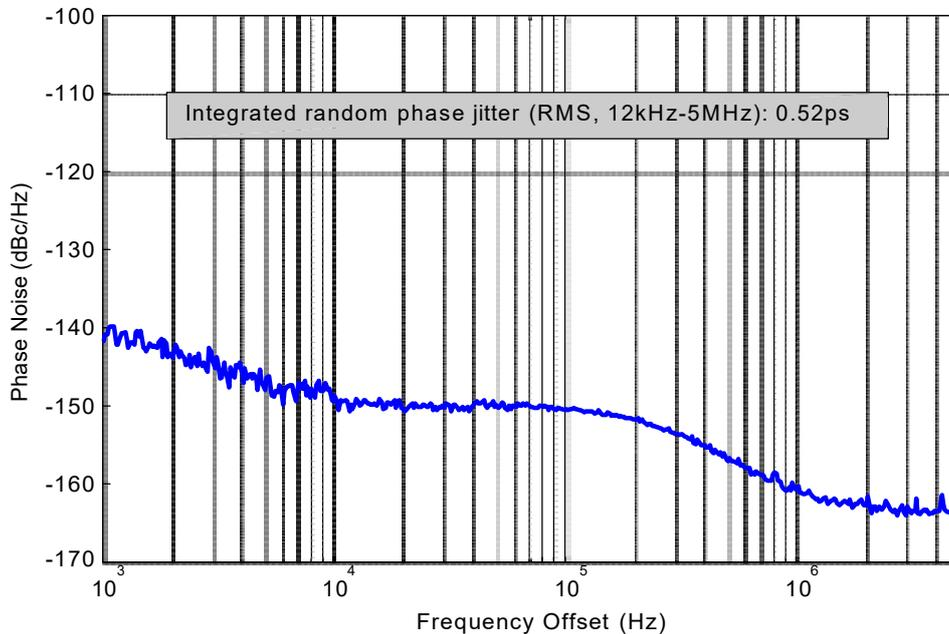
Figure 1. Phase Noise, 10 MHz, 3.3V, LVCMOS Output
