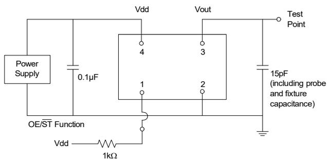
Figure 2. Test Circuit
