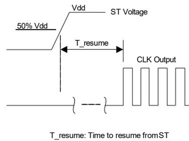
Figure 5. Standby Resume Timing ( $\overline{\text{ST}}$  Mode Only)
