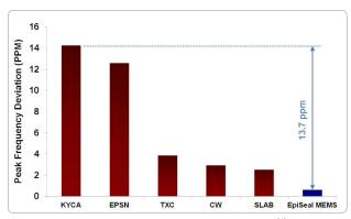
Figure 4. Power Supply Noise Rejection<sup>[4]</sup>
