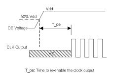
Figure 6. OE Enable Timing (OE Mode Only)
