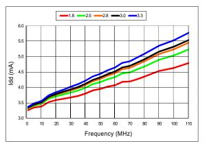
Figure 8. Idd vs Frequency
