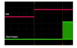
Figure 17. Startup Waveform vs. Vdd
