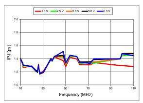
Figure 14. RMS Integrated Phase Jitter Random (12 kHz to 20 MHz) vs Frequency<sup>[9]</sup>
