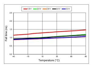
Figure 13. 20%-80% Fall Time vs Temperature
