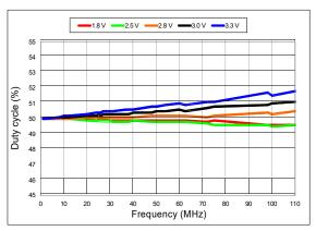
Figure 11. Duty Cycle vs Frequency
