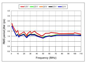
Figure 10. RMS Period Jitter vs Frequency
