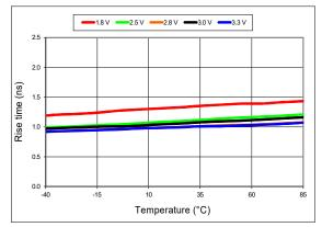
Figure 12. 20%-80% Rise Time vs Temperature
