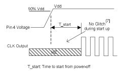
Figure 4. Startup Timing (OE/STMode)
