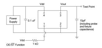
Figure 2. Test Circuit
