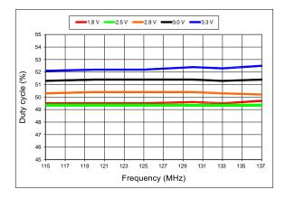
Figure 11. Duty Cycle vs Frequency
