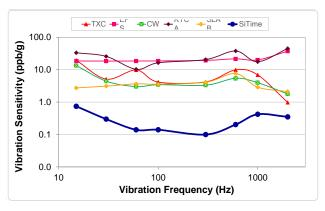
Figure 5. Vibration Robustness<sup>[5]</sup>
