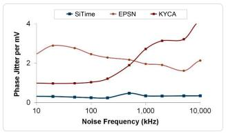
Figure 4. Power Supply Noise Rejection<sup>[4]</sup>
