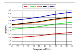
Figure 8. Idd vs Frequency
