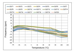
Figure 9. Frequency vs Temperature
