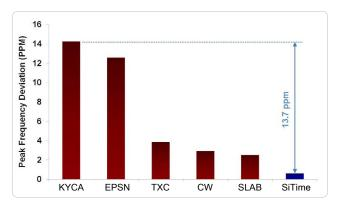
Figure 6. Shock Robustness<sup>[6]</sup>
