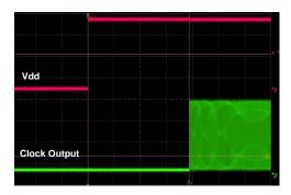
Figure 17. Startup Waveform vs. Vdd
