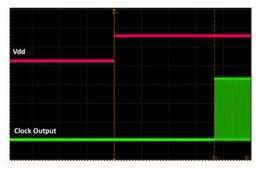
Figure 16. Startup Waveform vs. Vdd
