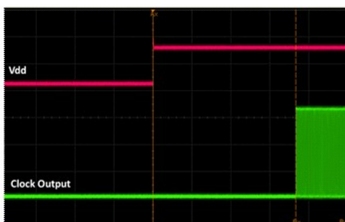
Figure 17. Startup Waveform vs. Vdd
