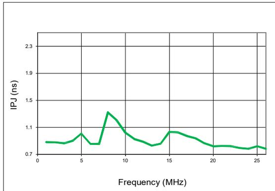
**Figure 14. RMS Phase Jitter Random vs Frequency<sup>[8]</sup>**
