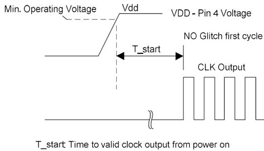
$T_{start}$ : Time to valid clock output from power on
