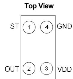
**Figure 1. Pin Assignments**
