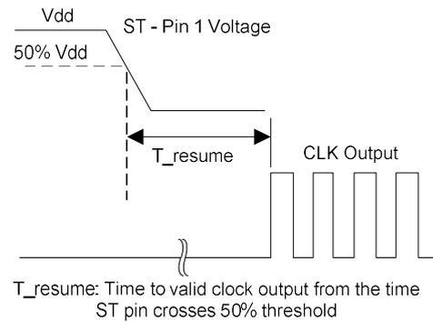
$T_{resume}$ : Time to valid clock output from the time ST pin crosses 50% threshold
