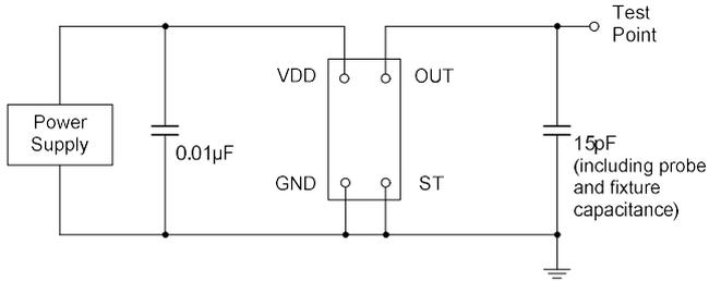
Figure 3. Test Circuit
