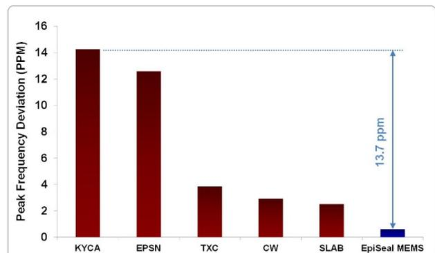
Figure 4. Power Supply Noise Rejection<sup>[4]</sup>
