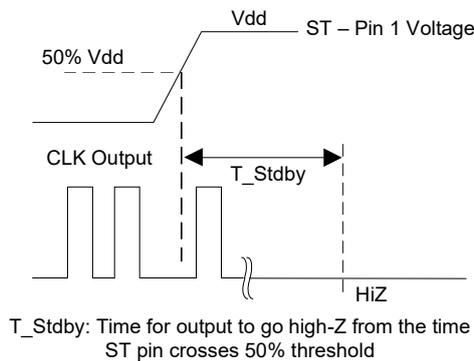
$T_{Stdby}$ : Time for output to go high-Z from the time ST pin crosses 50% threshold
