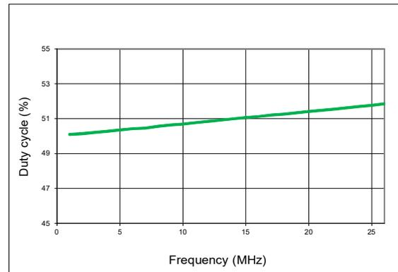
Figure 11. Duty Cycle vs Frequency
