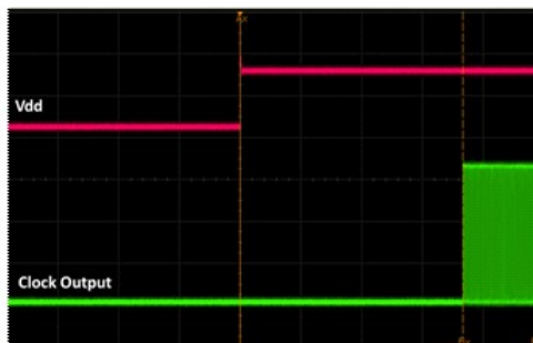
Figure 16. Startup Waveform vs. Vdd
