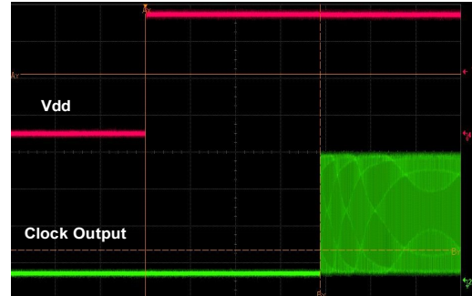
Figure 17. Startup Waveform vs. Vdd
