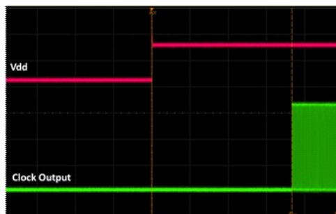
Figure 17. Startup Waveform vs. Vdd
