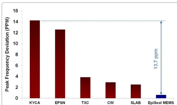
Figure 4. Power Supply Noise Rejection<sup>[4]</sup>
