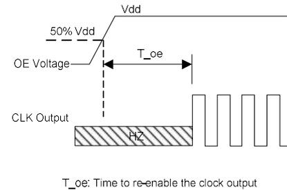
Figure 5. OE Enable Timing (OE Mode Only)
