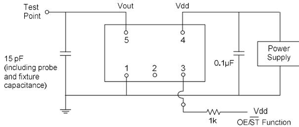
Figure 2. Test Circuit
