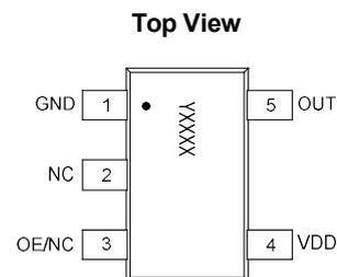
**Figure 1. Pin Assignments**
