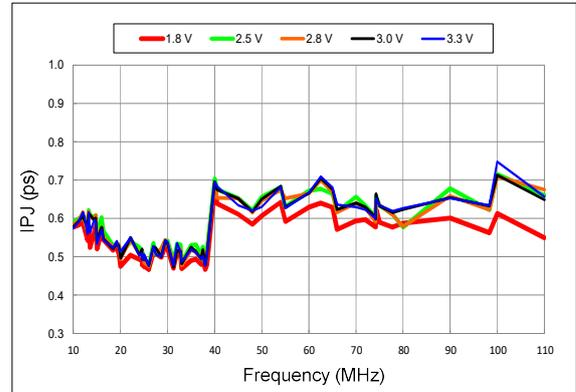
Figure 14. RMS Integrated Phase Jitter Random (900 kHz to 20 MHz) vs Frequency<sup>[9]</sup>
