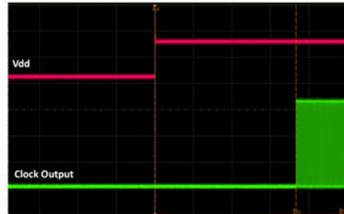
Figure 16. Startup Waveform vs. Vdd
